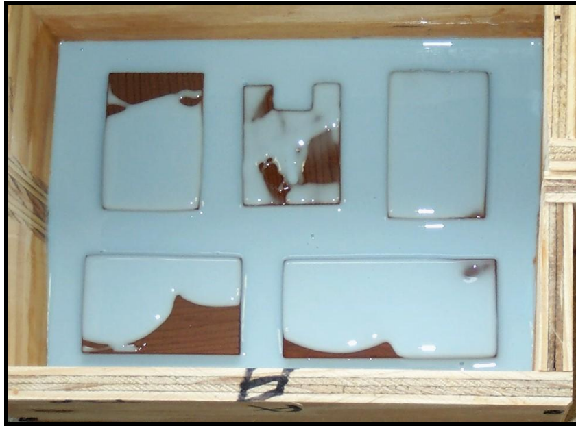
Silicone poured over spacers
