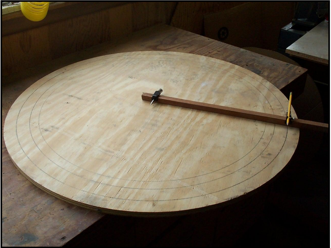
Use travel to lay out circles for pit wall
